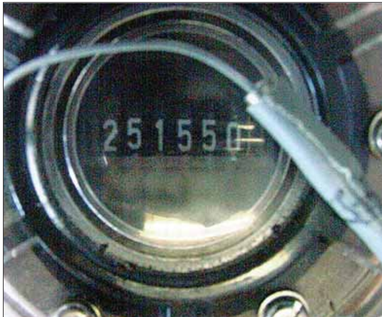
Interface valve performed more than 250,000 cycles
